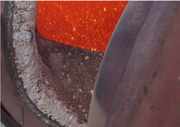
Photo 1-heavier particles are thrown in bed
