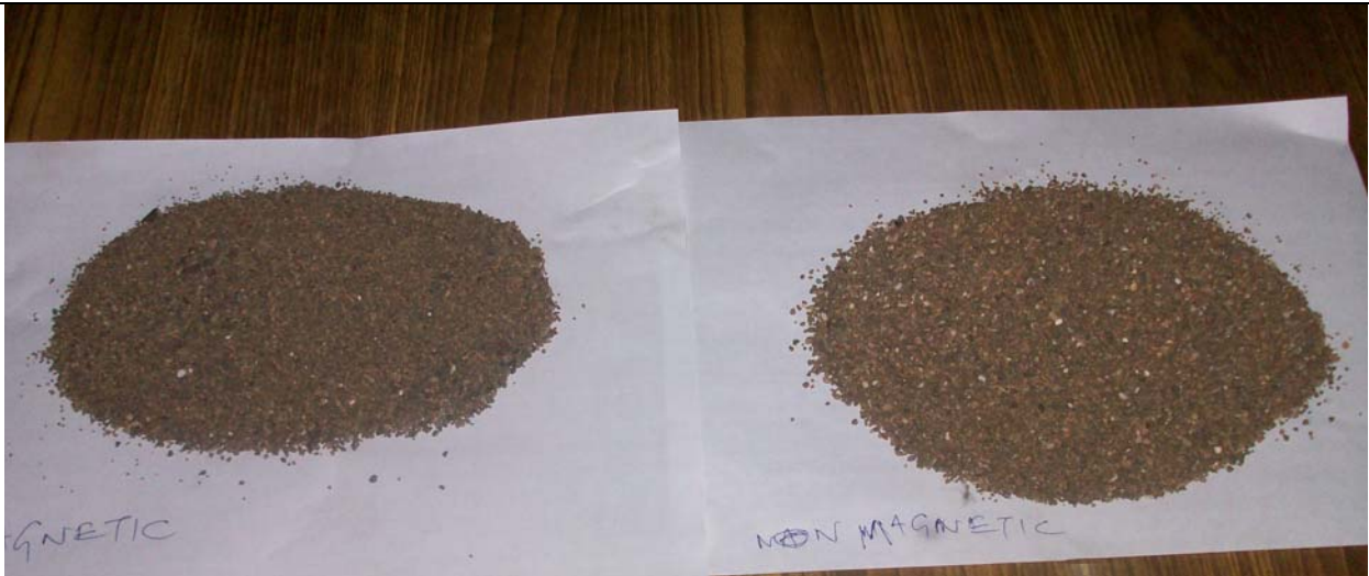
Photo 7: A sample of bed ash was checked in a boiler where the total bed defluidized due to iron containing bed ash particles. The weight % of iron containing particles is found to be 51.9%.
