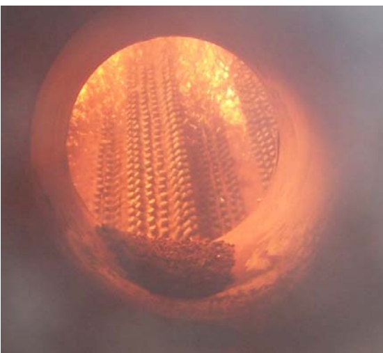
Photo 5-Improper fluidization –High DP drop
