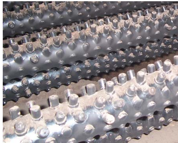
Photo 4- bed coil erosion in overbed fed boiler. The heavier particles settling at bottom of the bed has caused erosion.
